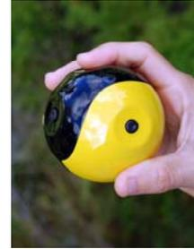
(Boston, MA — August 29, 2012) Boston-based inventor Steve Hollinger has been awarded U.S. Patent 8,237,787, “Ball with camera and trajectory control for reconnaissance or recreation.” Hollinger’s patent describes a throwable camera that employs an onboard position sensor to trigger image capture over the course of its airborne trajectory.
